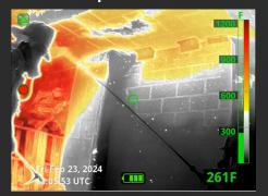
It's intuitive colorization. Kicking in at 500° F (260° C), this color threshold visually alerts firefighters when temperatures approach a range that may begin to damage personal protective equipment. Consistent and transparent color scheme for quick scene assessment.
